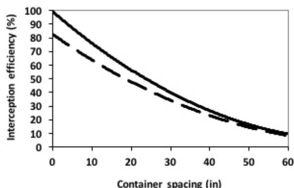
Figure 11. Effect of increased container spacing on interception efficiency for triangular (solid line) and square (dashed line) spaced containers.
