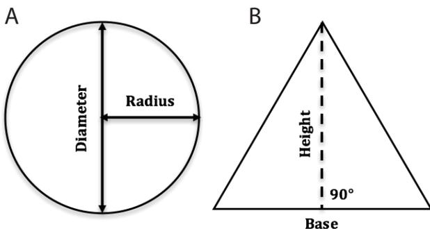
Figure 9. A, illustration of the diameter and radius of a circle; the area of a circle =  $\pi r^2$ , where  $\pi = 3.14$  and  $r =$  radius. B, the base and height of a triangle; the area of a triangle =  $0.5 b \times h$ , where  $b =$  length of the base and  $h =$  height.
