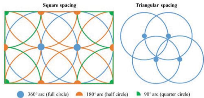
Figure 6. Overhead view of a hypothetical irrigation zone showing head-to-head coverage (each sprinkler reaches adjacent sprinklers) and typical sprinkler arcs for square and triangular sprinkler orientations.
