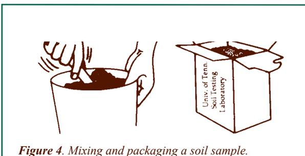
**Figure 4.** Mixing and packaging a soil sample.
