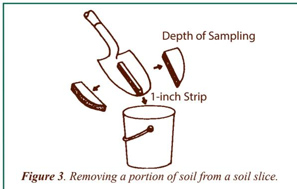
**Figure 3.** Removing a portion of soil from a soil slice.
