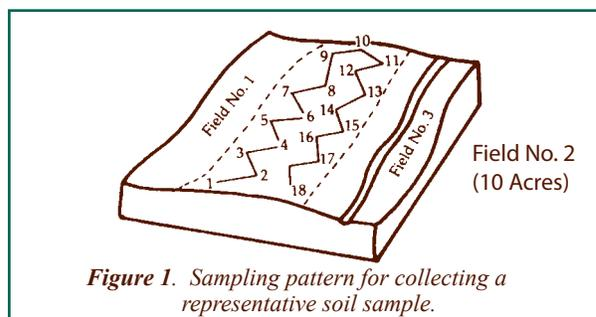
Figure 1. Sampling pattern for collecting a representative soil sample.
